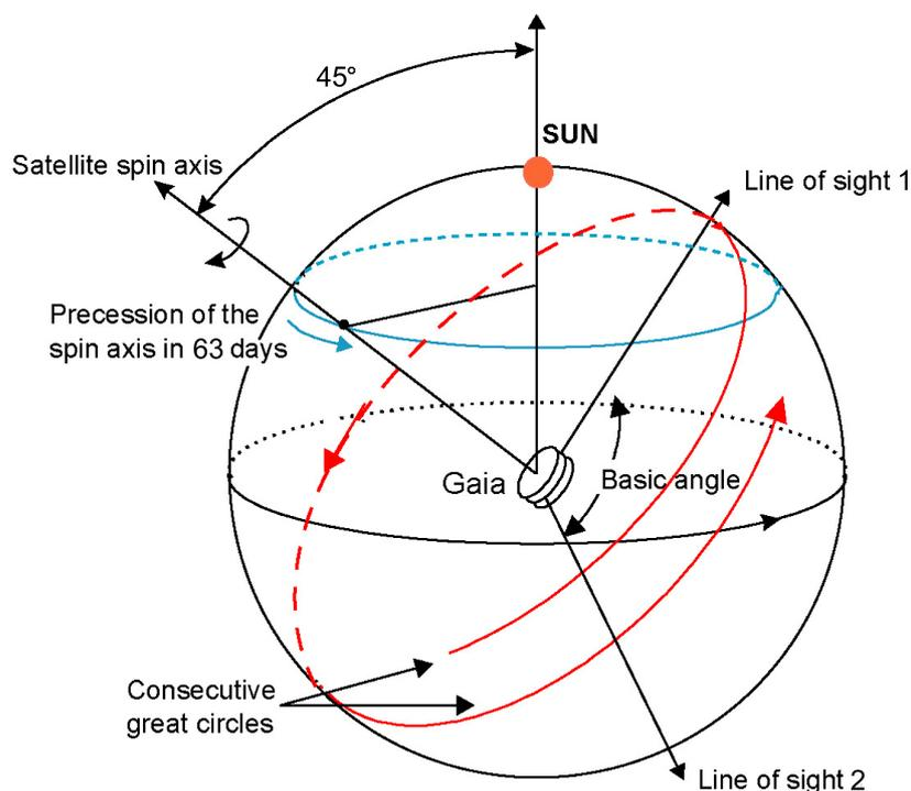
Gaia's two astrometric fields of view scan the sky according to a carefully prescribed 'revolving scanning law'. The constant spin rate of  $60 \text{ arcsec s}^{-1}$  corresponds to 6-hour great-circle scans. The angle between the slowly precessing spin axis and the Sun is maintained at  $45^\circ$ . The basic angle is  $106.5^\circ$ .
